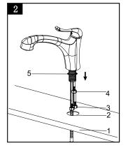
Drill a  $\emptyset$ 1-3/8"to  $\emptyset$ 1-1/2" hole (2) in sink (1) Put rubber gasket(5) into base groove and then insert the faucet through the hole (2).
