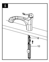
Connect the hose (10) with outlet pipe (4).
