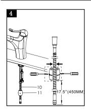
Fix weight balance(11) on the suitable position of sprayer flexible hose (10) to keep the pulling smoothly. The distance from the end of the outlet pipe connector to the weight balance should be 17.5".
