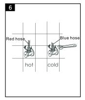
Connect the flexible hoses to the Water-supplying value (left to hot water and right to cold)
