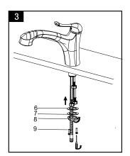
Put all hose through the plastic gasket (6) then through the metal washer (7), finally screw the locking nut (8), tight it with (9).
