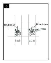
Connect the flexible hoses to the Water-supplying value (left to hot water and right to cold)
