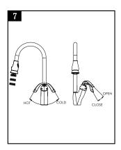
Move the handle rightward or Leftward in counterclockwise from cold the hot.
