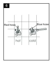
Water-supplying value(left to hot water and right to cold)
