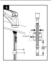
Fix weight balance (9) on the suitable position of sprayer flexible hose (8) to keep the pulling smoothly. The distance from the end of the outlet pipe connector to the weight balance should be 30".
