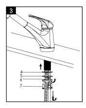
Put all hose through the rubber gasket (4) then through gasket (5), finally screw the nut fitting (6), tight it with (7).
