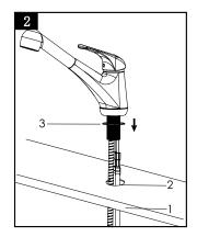
Drill a  $\emptyset$ 1-3/8" hole (2) in sink (1) . Put O-ring (3) into base groove and then insert the faucet through the hole(2)
