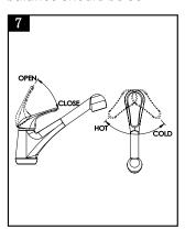
Pull the handle up to turn on the faucet, push down to horizontal line to close. Move the handle left to control the hot water, move the handle right to control the cold water.
