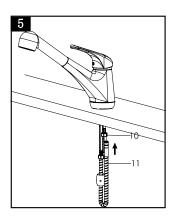
Connect the hose (11) with outlet pipe (10)
