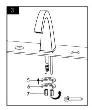
Adjust the faucet to the right position and put on the rubber washers (5) and mental washer (6) and tighten tightly with nuts(7).
