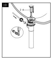
As shown, place the drain stopper (24)into the drain rod into the ball rod opening through stopper hole, and threaded it.
