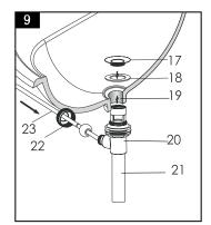
Insert flange(17) with washer (18) through sink drain Hole(19). Then thread the drain body(20) into the flange from under. Holding the drain body(20) in position with ball rod (23) opening facing back. Tighten the lock nut(22). Finally thread drain tailpiece (21) into drain body.
