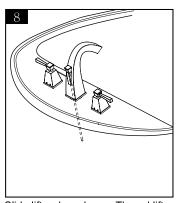
Slide lift rod as shown. Thread lift rod into lift knob.
