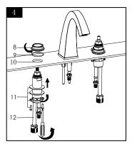
Put the b cknut(8)p -ring(9) on thev alve body(12) successively. Put the valveb ody (12) through the Ø28 mm hole (11) from under. Andti ght he I ocknut((8).
