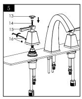
Connect the handle body(15) tightly it by screw(16). Put the screw (14) under the ornament cover (13) and install the cover on the handle.
