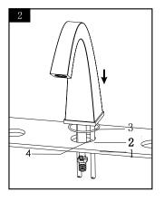
Drill a  $\emptyset 33$ mm hole (2) in sink (1). Install the fixing rod(4)and and screw them firmly . Put O-ring (3) into base groove and then insert the them through the hole(2).
