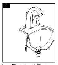
Insert lift rod through lift rod strap and secure with set screw. Place the ball rod through one of the holes on the lift rod strap. Secure if With the spring clip.
