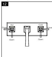
Turn the left handle counter clock wise to get the hot water, turn the right handle clockwise to get the cold water.
