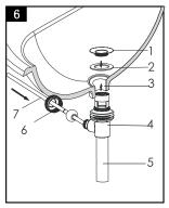
As shown, insert flange(1) with washer (2) through sink drain hole (3). Thread drain body (4) in position with ball rod(7) under from the opening facing back, tighten metal locknut(6) securely. thread drain tailpiece(5) into drain body.
