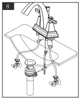
Insert lift rod through lift rod strap and secure with set screw. Place the ball rod through one of the holes on the lift rod strap. Secure it with the spring clip.
