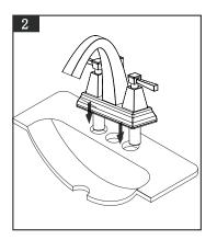
Drill three  $\emptyset$ 28mm holes on the sink. Install the body into the holes.
