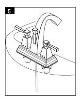
Slide lift rod as shown. Thread lift rod into lift knob.
