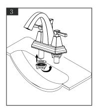
Put the rubber washer and locking nut on, Wrench up the locking nut to lock the faucet on sink.
