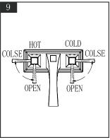
Turn the left handle counterclockwise to get the hot water. turn the right handle clockwise to get the cold water.
