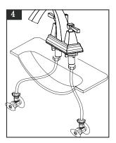
Connect the two flexible hoses to water supply valves.
