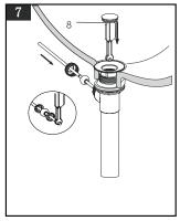
As shown, place the drain stopper (8) into the drain rod into the ball rod opening through stopper hole and threaded it.
